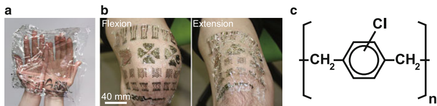
Fig. 6.10 Fully printed organic circuits fabricated on ultrathin substrate. (a) A photograph of organic TFT devices on 1-mm-thick parylene-C films. (b) Organic device films conforming to a human knee. Our devices were fabricated entirely by printing, enabling them to be easily fabricated on a large scale, which can cover whole area of a human skin as shown in (b). (c) The chemical structure of parylene-C (Adapted from Ref. [33]. Copyright 2014, Nature Publishing Group)
