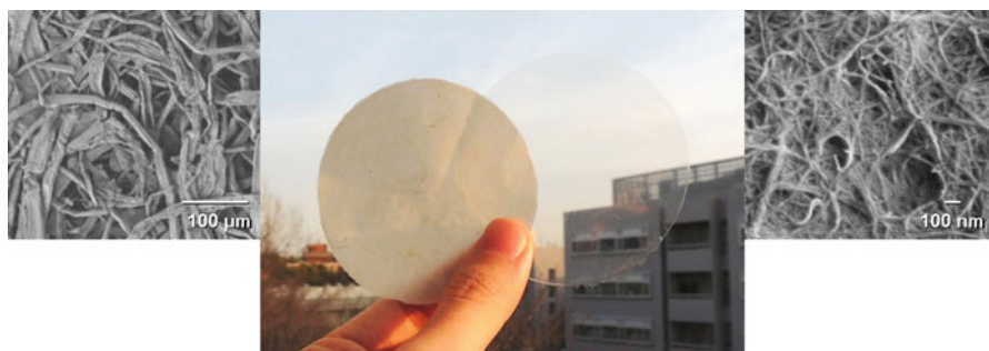
Fig. 4.1 Optical and SEM images of conventional cellulose paper made from pulp fibers with a width of tens of \mu\text{m} ( left ) and optically transparent nanofiber paper made from cellulose nanofibers with a width of ca. 15 nm ( right )
